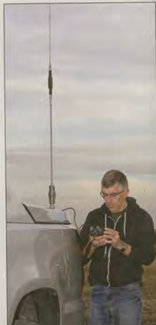
The author measuring the impedance of his 17 meter band antenna.
